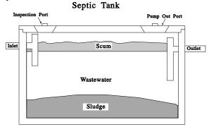
Tees, or baffles, are provided at the tank's inlet and outlet pipes. The inlet tee slows the incoming wastes and reduces disturbance of the settled sludge. The outlet tee keeps the solids and scum in the tank. As new wastewater enters the tank through the inlet tee, an equal amount of wastewater is pushed out of the tank through the outlet tee. The effluent that leaves the tank has been partially treated but still contains disease-causing bacteria and other pollutants.
